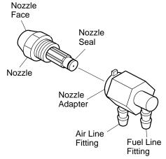
Figure 15 - Nozzle and Nozzle Adapter
