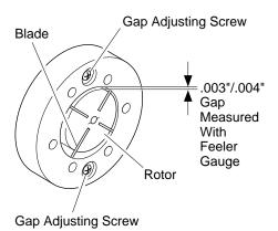
Figure 18 - Gap Adjusting Screw Locations
