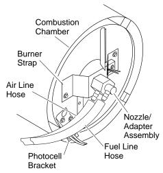
Figure 12 - Removing Air and Fuel Line Hoses (110,000 and 115,000 Btu/Hr Models Only)
