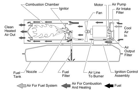
Figure 3 - Cross Section Operational View
