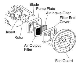
Figure 17 - Rotor Location
