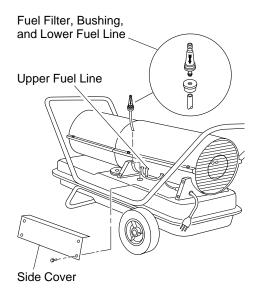
Figure 9 - Fuel Filter Removal
