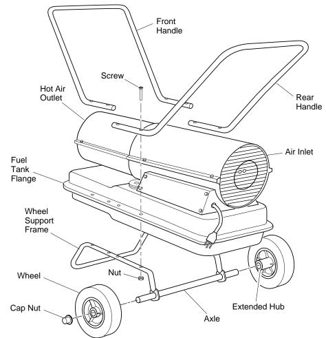
Figure 2 - Wheel and Handle Assembly
