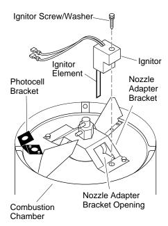
Figure 11 - Ignitor Replacement
