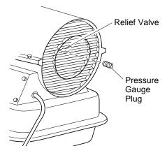
Figure 7 - Pressure Gauge Plug Removal
