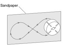
Figure 19 - Sanding Rotor
