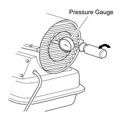
Figure 8 - Adjusting Pump Pressure
