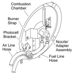
Figure 13 - Removing Air and Fuel Line Hoses (150, 155, and 165,000 Btu/Hr Models Only)
