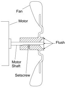
Figure 5 - Fan Cross Section
