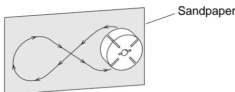
**Figure 19 - Sanding Rotor**
