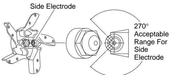
**Figure 14 - Acceptable Range For Side Electrode**
