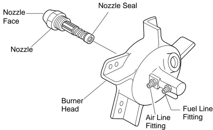
**Figure 16 - Removing Nozzle**
