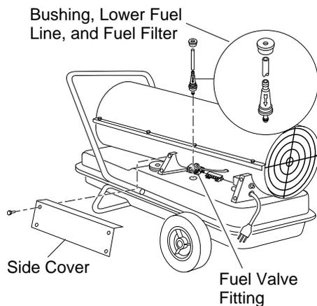
**Figure 10 - Fuel Filter Removal**
