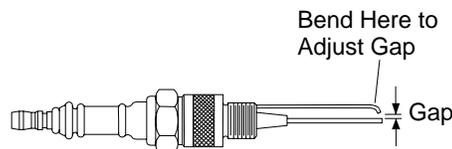
**Figure 13 - Spark Plug Gap**
