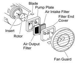
Figure 16 - Rotor Location
