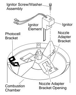
Figure 11 - Ignitor Replacement
