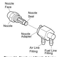
Figure 14 - Nozzle and Nozzle Adapter
