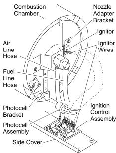
Figure 10 - Disconnecting Ignitor Wires from Ignition Control Assembly
