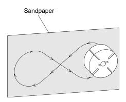
Figure 18 - Sanding Rotor
