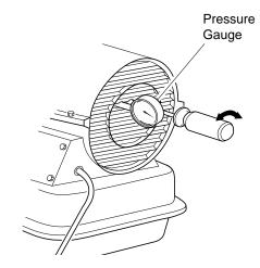
Figure 8 - Adjusting Pump Pressure
