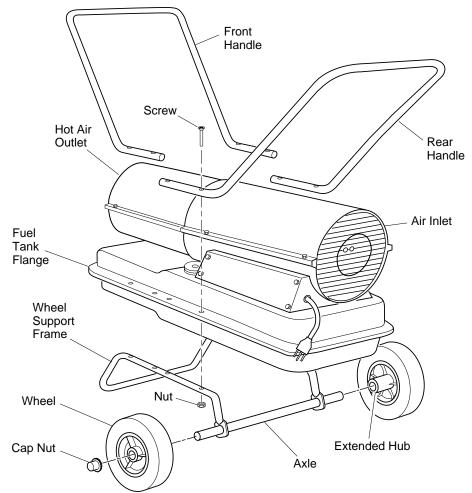
Figure 2 - Wheel and Handle Assembly
