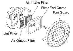
Figure 6 - Air Output, Air Intake, and Lint Filters
