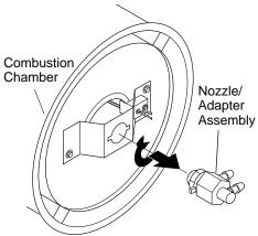
Figure 13 - Removing Nozzle/Adapter Assembly
