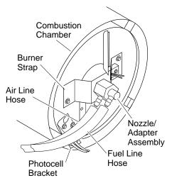
Figure 12 - Removing Air and Fuel Line Hoses
