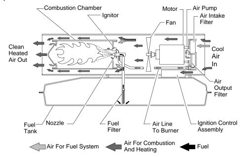
Figure 3 - Cross Section Operational View
