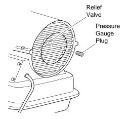
Figure 7 - Pressure Gauge Plug Removal
