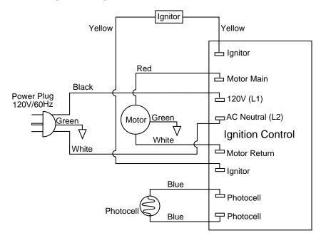
Figure 20 - Wiring Diagram
