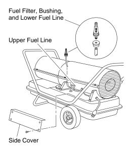
Figure 9 - Fuel Filter Removal
