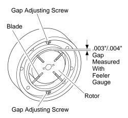
Figure 17 - Gap Adjusting Screw Locations
