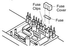
Figure 19 - Replacing Fuse
