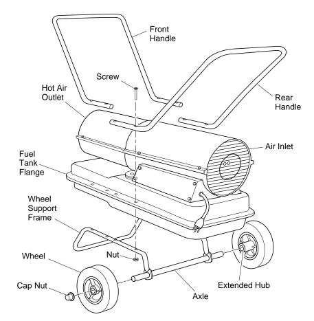
Figure 2 - Wheel and Handle Assembly
