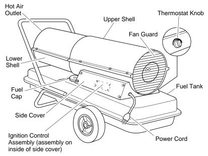
Figure 1 - Portable Forced Air Heater
