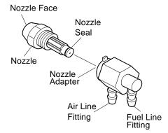
Figure 14 - Nozzle and Nozzle Adapter
