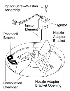
Figure 11 - Ignitor Replacement
