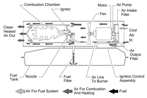
Figure 3 - Cross Section Operational View
