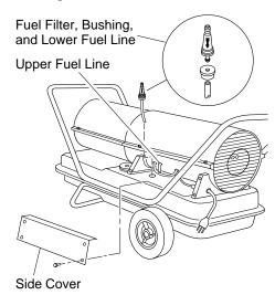
Figure 9 - Fuel Filter Removal
