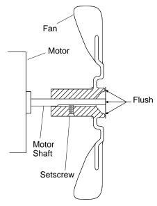
Figure 5 - Fan Cross Section
