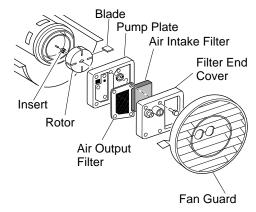
Figure 16 - Rotor Location
