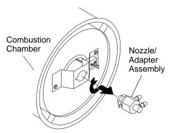
Figure 13 - Removing Nozzle/Adapter Assembly
