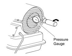
Figure 8 - Adjusting Pump Pressure
