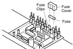
Figure 19 - Replacing Fuse
