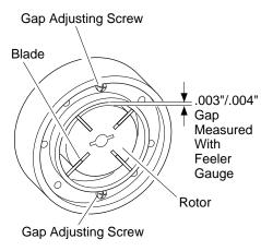
Figure 17-Gap Adjusting Screw Locations
