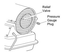
Figure 7 - Pressure Gauge Plug Removal
