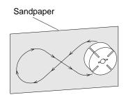
Figure 18 - Sanding Rotor
