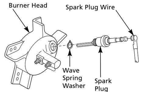
Figure 13 - Spark Plug Removal
