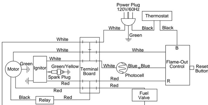
Figure 26 - Wiring Diagram
