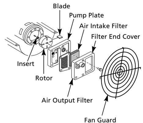
Figure 18 - Rotor Location
