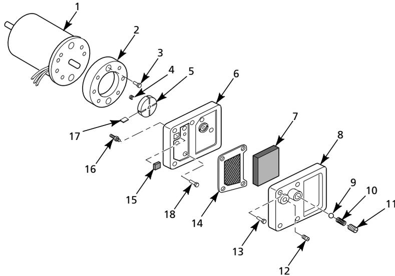
**Figure 21 - Motor and Pump Assembly**
