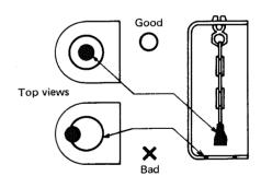
4. Open the access door and center the wire handle in the opening. If the handle is not visible, turn the heat chamber untill you can grasp the handle. Be sure that by moving the wire handle left and right, the heat chamber moves easily. This means that the heat chamber is properly seated.
