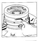
5. Slide the rubber packing off the wick. If the rubber packing remains on the tank, remove the packing from the tank.
