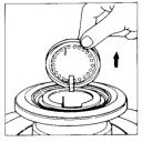
Push the Igniter lever to raise the igniter coil into view.
