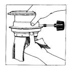
9. Slide the rubber packing over the bottom of the wick and install it on the wick adjuster. Insert the projection on the packing into the hole on the rear of the adjuster. Be sure the four (4) tails of the wick extend downward.
