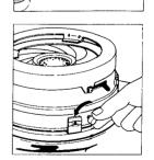
Pull the reset lever toward you about two (2) inches. This opens the extinguisher shutter enough to clear the igniter cover. Lift off the extinguisher assembly.
