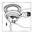
8. Fold the new wick and insert it into the wick adjuster. Align the bottom of the orange guide strip on the outside of the wick with the bottom of the wick adjuster.
