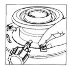
Wick height should be 8 mm (5/16 in.) when wick adjuster knob is fully clockwise. Be sure to check.
