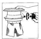
7. Fold the wick in towards the center to free it from the wick adjuster and then remove the old wick.
