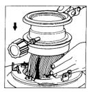
The space between the wick adjuster and the primary air tube should be even all around.
