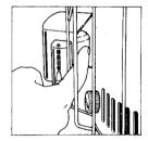
2. Remove the three (3) LARGE thumbscrews holding the outer cover. Lift off the cover with the carrying handle.
