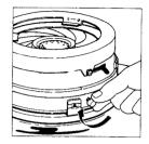
12. Replace the outer cover on the fuel tank and secure it into position with three (3) LARGE thumbscrews. Replace the batteries in the battery holder.
