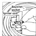
Note that the igniter coil fits into the bayonet socket the same way a flashlight bulb fits into its holder. To remove the igniter coil, push it in and twist it in either direction while holding the sides of the socket with your other hand. Install the new igniter coil by pressing it into the socket and turning.
