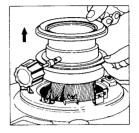
5. Slide the rubber packing off the wick. If the rubber packing remains on the tank, remove the packing from the tank.
