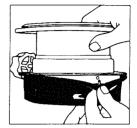
10. Lower the wick adjuster assembly into the fuel tank, guiding the four (4) tails of the wick so it fits over the primary air tube and evenly into place. Position the wick adjuster shaft in the U-shaped guide at the front of the tank.
