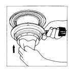
Finally, gently press the wick, all along its circumference, against the adjuster to insure that it is firmly in place.
