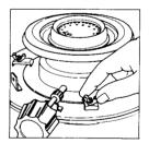
Wick height should be 7 mm (9/32 in.) when wick adjuster knob is fully clockwise. Be sure to check.
