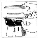
6. Turn the wick adjuster knob counterclockwise until it stops. Then gently pull the knob and continue turning counterclockwise to the lowest wick position.
