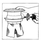
7. Fold the wick in towards the center to free it from the wick adjuster and then remove the old wick.
