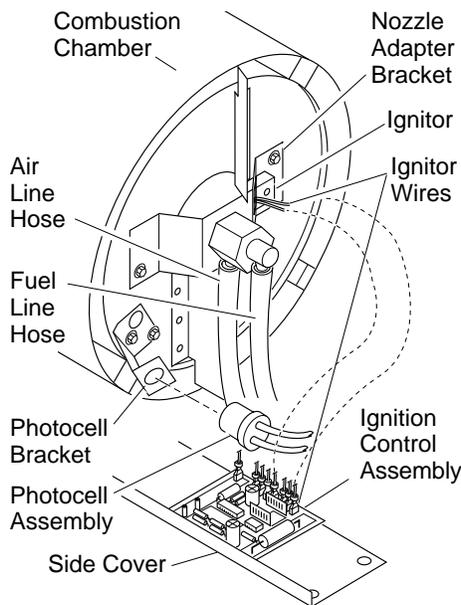
**Figure 10 - Disconnecting Ignitor Wires from Ignition Control Assembly**
