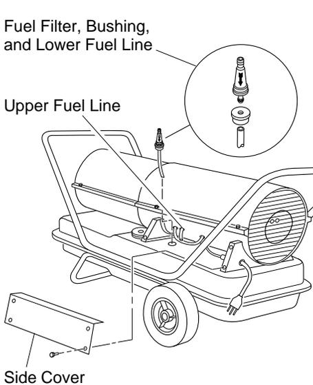
**Figure 9 - Fuel Filter Removal**
