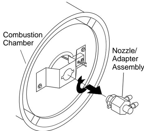
**Figure 13 - Removing Nozzle/Adapter Assembly**
