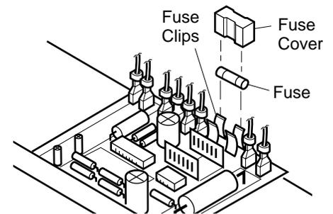
**Figure 19 - Replacing Fuse**
