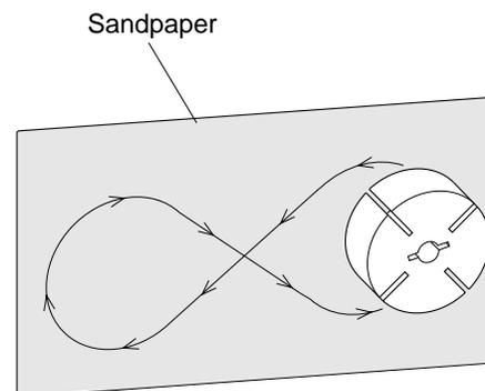
**Figure 18 - Sanding Rotor**
