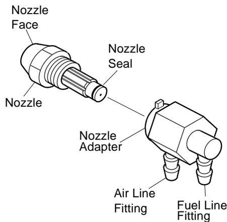
**Figure 14 - Nozzle and Nozzle Adapter**
