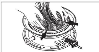
**NOTE** : Turn the Wick adjustment Knob and check that the Wick moves up and down.
