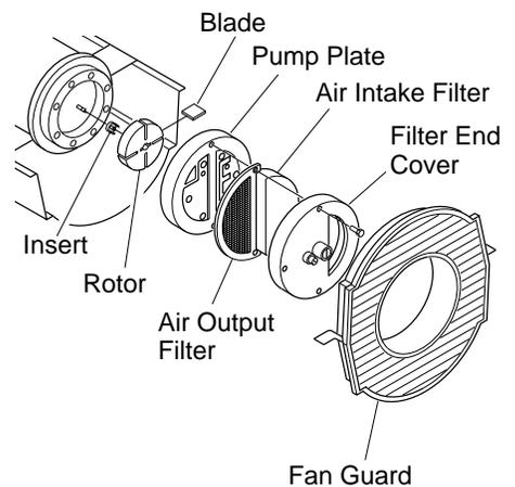
**Figure 15 - Rotor Location**
