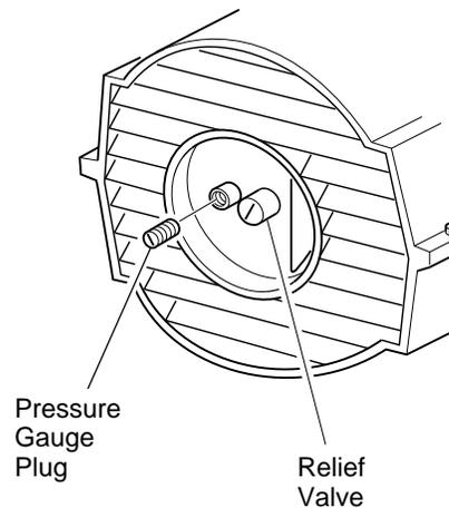
**Figure 6 - Pressure Gauge Plug Removal**
