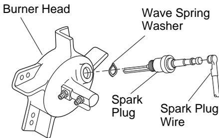
**Figure 12 - Spark Plug Removal**
