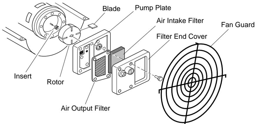
**Figure 17 - Rotor Location**
