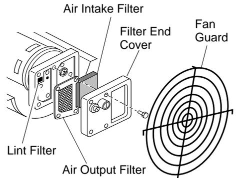
Figure 7 - Air Output, Air Intake, and Lint Filters
